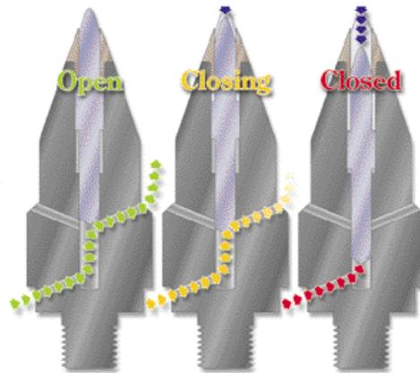
*Unlike the 30-year-old technology valves which close by flow, the Repeater™ Valve closes via pressure. This gives the molder an amazing amount of precision and control.*
